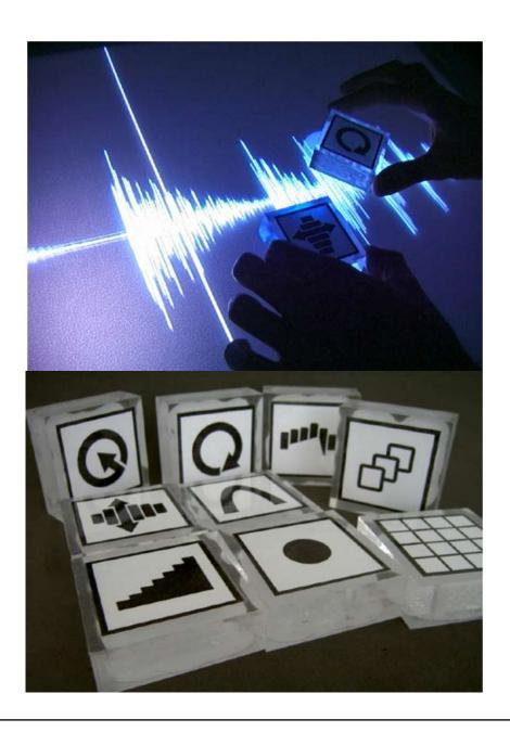
Prototype design and programming of a sound editor with a tangible interface. Developed together with Gerard Roma with the support of the MTG.
