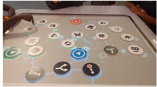
Figure 5. A group creating an audiovisual piece with the TuneTable using 3 play() blocks, 2 go-to() blocks, a conditional() block, a split() block, and 14 sound() blocks.
